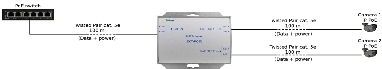
Connection of two IP PoE cameras and extension of the range for another 100m
